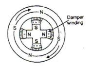
In electrical engineering, a synchronous condenser are sometimes called a synchronous or synchronous compensator
