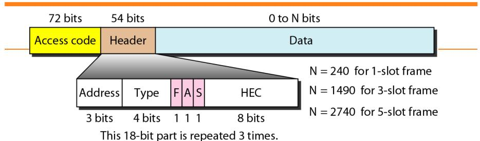
Access code: 72-bit field normally contains sync bits and ID of the primary to distinguish the frame of one piconet from another
