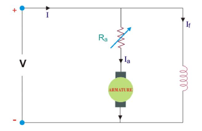
Derive the voltage equation for DC Shunt Motor
