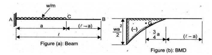
Bending moment diagram for the given beam is shown in figure (b).
