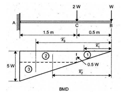
The Bending moment diagram is shown in Fig (b).
