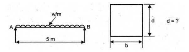
$\Delta_{max} = y_{center} = 10 \text{ mm};$ E = 1.2 × 10<sup>4</sup> N/mm<sup>2</sup> (f<sub>b</sub>)<sub>max</sub> = 8 N/mm<sup>2</sup>; 1 = 5m = 5000 mm
