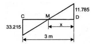
Let the point of zero shear force (or maximum BM) occurs at M, at a distance of x from D. Now, from similar triangles,
