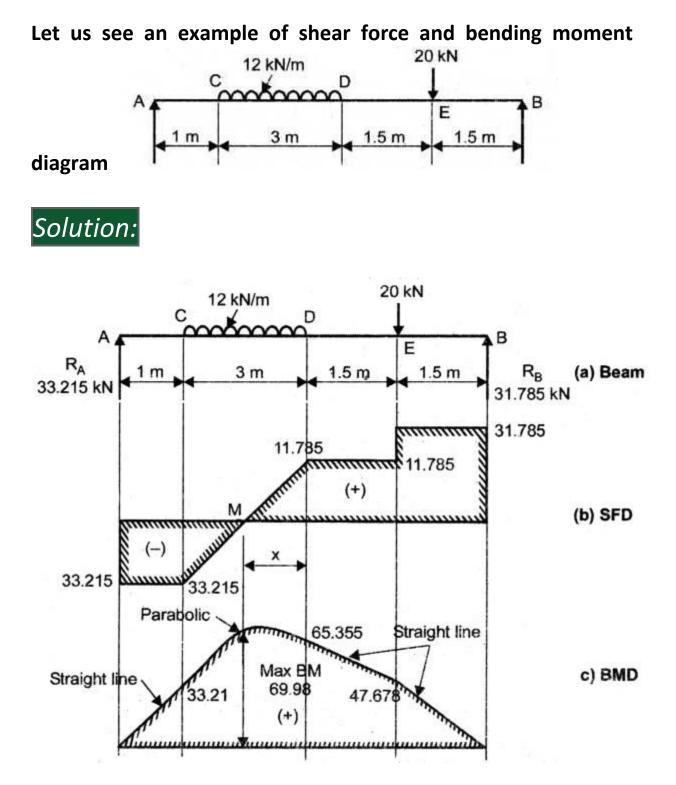
Given beam is simply supported. Hence support reactions are to be determined before finding Shear force and Bending moment values at various points.  $Let R_A$  = Reaction at  $A R_B$  = Reaction at B
