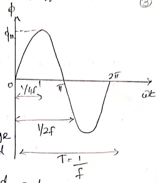
From Faraday's Law of electromagnetic induction the average emf induced in each turn is  $\propto$  to the average rate of change of flux.
