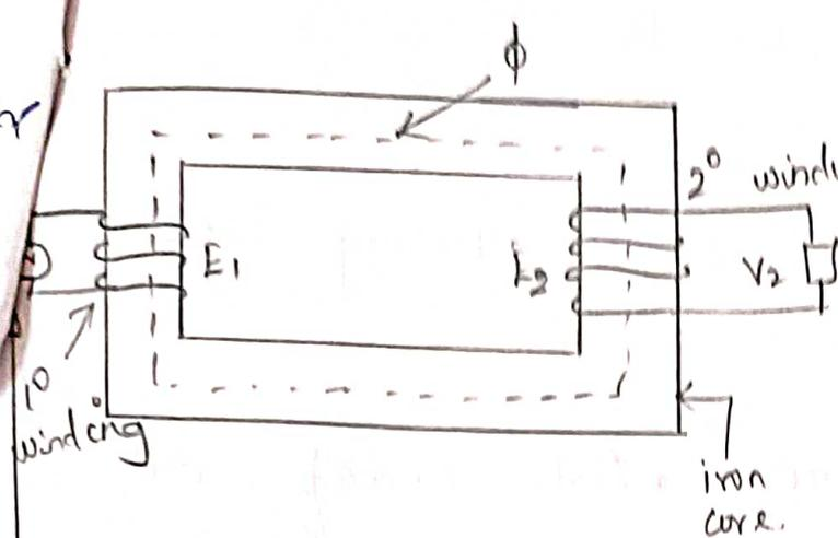
A transformer operates on the principle of mutual inductance b/w two inductively coupled coils.
