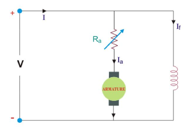
Derive the voltage equation for DC Shunt Motor
