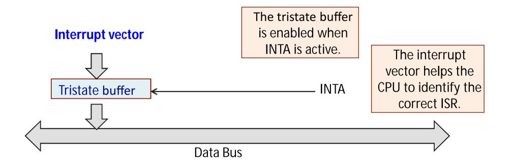
•A common solution is to use a priority interrupt controller.
