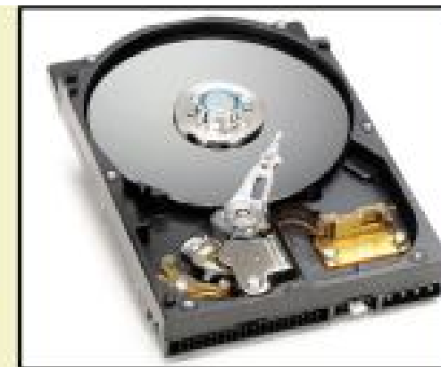
3.5" magnetic disk (1 Tbytes)
