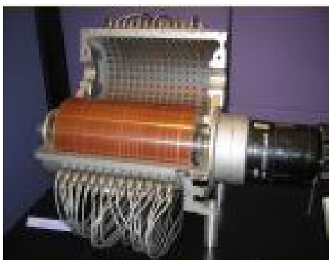
Magnetic drum (62.5 Kbytes)
