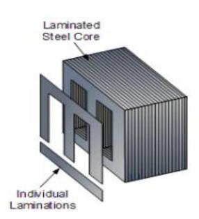
> Laminated sheets of steel are used to reduce eddy current loss.(I^2R Loss)
