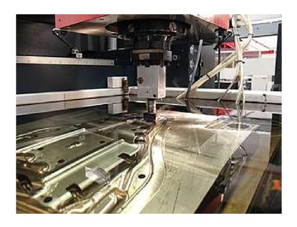
Material is removed from the work piece by a series of rapidly recurring current discharges between two <u>electrodes</u>, separated by a <u>dielectric</u> liquid and subject to an electric <u>voltage</u>. One of the electrodes is called the tool-electrode, or simply the *tool* or *electrode*,
