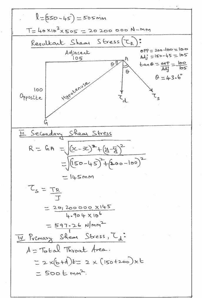
$$T_{d} = \frac{P}{A} = \frac{40,000}{500t} = \frac{80}{t} \text{ N/mm}^{2}.$$
