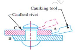
In order to make the joints leak proof or fluid tight in pressure vessels like steam boilers, air receivers and tanks etc. a process known as caulking is employed. In this process, a narrow blunt tool called caulking tool, about 5 mm thick and 38 mm in breadth,
