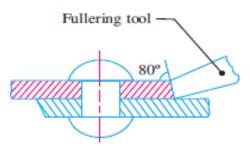
fullering which has largely superseded caulking. In this case, a fullering tool with a thickness at the end equal to that of the plate is used in such a way that the greatest pressure due to the blows occur near the joint, giving a clean finish, with less risk of damaging the plate. A fullering process is shown in Fig.
