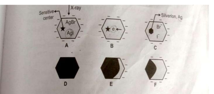
FIG. 7.7: Latent image formation: (A) X-ray exposure provide electrons, (B) electrons moves to the sensitive center, (C) mobile silver atoms moves to the sensitivity center combine with electron and forms latent image, (D) process repeated, latent image widens, (E) additional silver formation during processing, and (F) final metallic silver image
