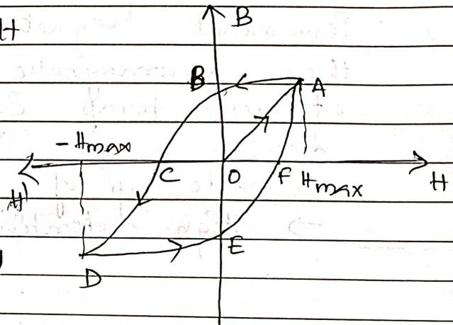
Through out the cycle, mag. induction  $\vec{B}$  lags behind magnetising field  $H$ . This lagging of  $B$  behind  $H$  is called hysteresis.
