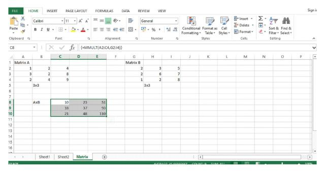
Fig 9: Matrix Multiplication using MMULT () Function
