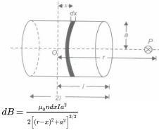
where a is the radius of loop, n is the number of turns per unit length of solenoid and r is the distance of point from the centre of a solenoid.
