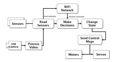
The preceding diagram illustrates how we have instantiated the OODA loop into the software and hardware of our robot. The robot can either act autonomously, or accept commands from a control station connected via a wireless network.
