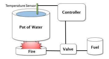
The Valve controls the heat produced by the fire, which warms the pot of water. The Temperature Sensor detects if the water is too cold, too hot, or just right. The Controller uses this information to control the valve for more heat. This type of schema is called a closed loop control system.
