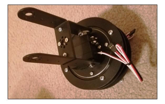
Now, all of the servos that attach to the C-shaped arms will go together the same way. We grab one of the small bearings and a short screw and fasten the bearing into the side of the rounded part of the C bracket away from the side of the servo. Now attach the
