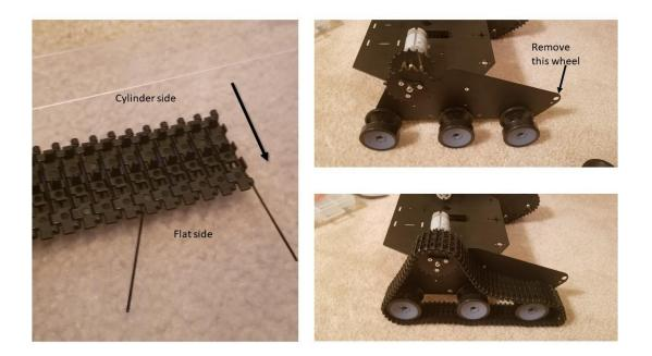
Now we can assemble the other large base plate on the bottom two holes in the track plates and our drive base is complete. The second base plate goes upside down relative to the first plate – the bent outer section goes up. I staggered the two plates by rotating the bottom plate 180 degrees, but they can also go exactly parallel if you want. I liked the staggered arrangement for later placement of sensors.
