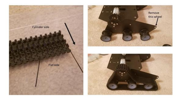
Now we can assemble the other large base plate on the bottom two holes in the track plates and our drive base is complete. The second base plate goes upside down relative to
