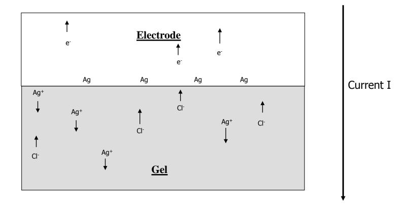
Illustrative diagram of electrode-electrolyte interface in case of Ag-AgCl electrode
