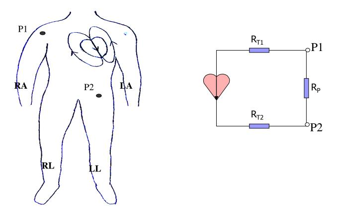
Points P1 and P2 are arbitrary observation points on the torso;  $R_{\rm P}$  is the resistance between them, and  $R_{\rm T1}$ ,  $R_{\rm T2}$  are lumped thoracic medium resistances.
