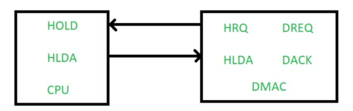
**2.** Cascade Mode – In this multiple channels are used, we can further cascade more number of DMACs.
