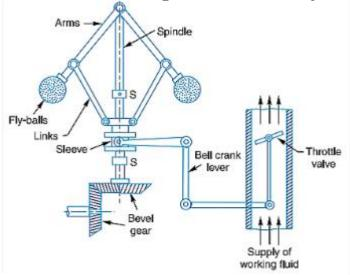
The basic principle of working of governor is that the governor spring and flyweights are so selected that at any designed engine speed centrifugal force and spring force are in equilibrium.
