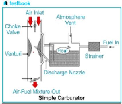
The float chamber supplies fuel to the main nozzle through the main fuel jet. Air is drawn into the carburettor from the atmosphere through the choke valve and passes through the venturi, which reduces the cross-sectional area of the airflow and increases its velocity.
