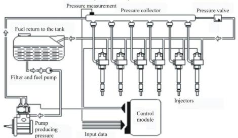
A high-pressure pump pressurises the fuel. A pressure regulating valve is attached to the high-pressure pump which gets input from ECU. The ECU receives signals from the throttle position sensor, temperature sensor, speed sensor and manifold pressure sensor.
