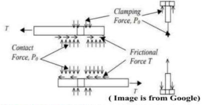
Only when the externally applied force exceeds the frictional resistance between the plates, the plates slip and the bolts bear against the bolt holes. Thus even after slip, there is a reserve strength due to bearing.
