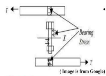
• The force is transferred by bearing between the plate and bolts at the bolt holes. The bolts experience single or double shear depending upon the plate configuration. The failure may be either by shearing of the bolts or bearing of the plate and the bolt.
