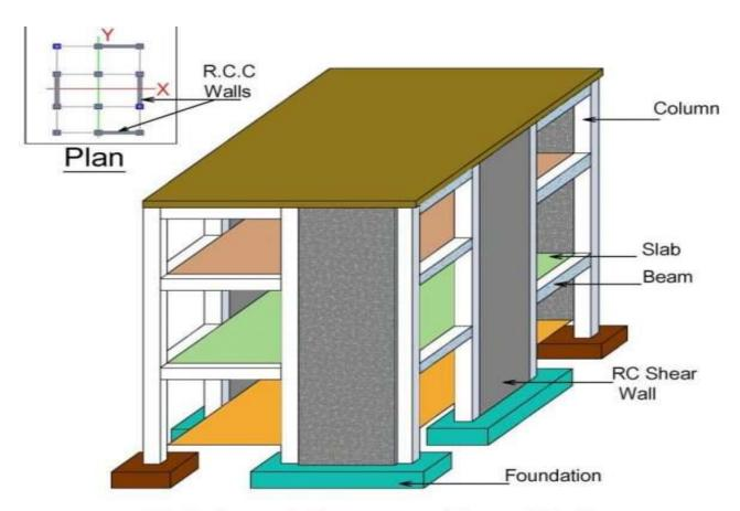
Reinforced Concrete Shear Wall
