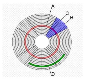
Figure 5: Data Arrangement on DIsk
