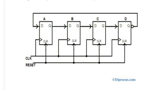
Consider the 4-bit Johnson counter, it contains 4 D flip-flops, which is called 4-bit Johnson counter. It has preset and clear pins to initialize or start and reset the counted.
