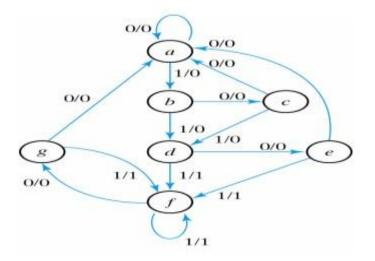
There are an infinite number of input sequences that may be applied; each results in a unique output sequence. Consider the input sequence 01010110100 starting from the initial state a:
