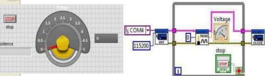
Interfacing a 10KΩ Potentiometer with LabView using Arduino Uno
