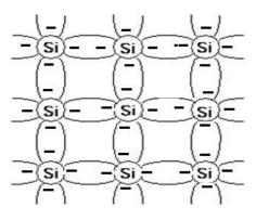
a hole which also acts as current carrier. These electrons and holes move in opposite directions under the effect of external field and constitute current.
