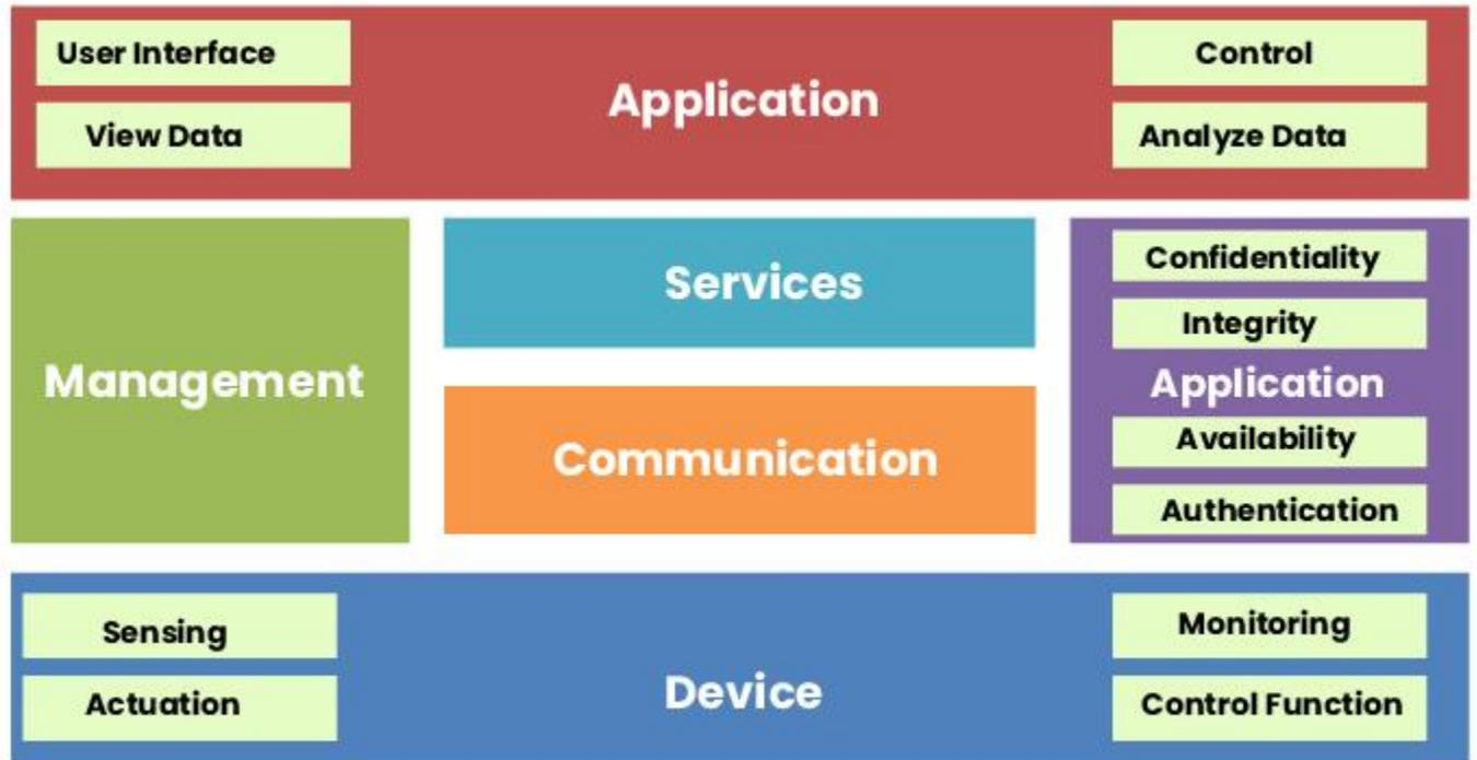
It is the actual design of the IoT system. It illustrates the assembling and configuration of the components i.e. computers, sensors, and actuators.
