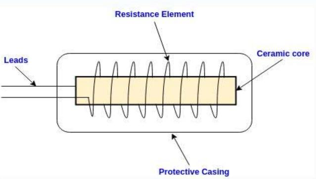
Copper, Nickel and Platinum are the most used RTD materials. These metals have positive temperature co-efficient and possess poor thermal sensitivity. Also, the resistance-temperature characteristics of these materials are approximately linear.
