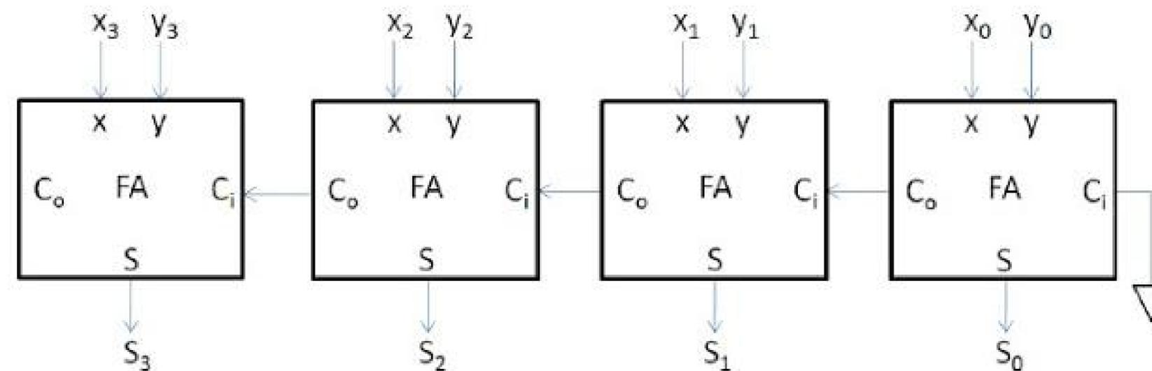
The 4-bit ripple-carry adder is built using 4 1-bit full adders
