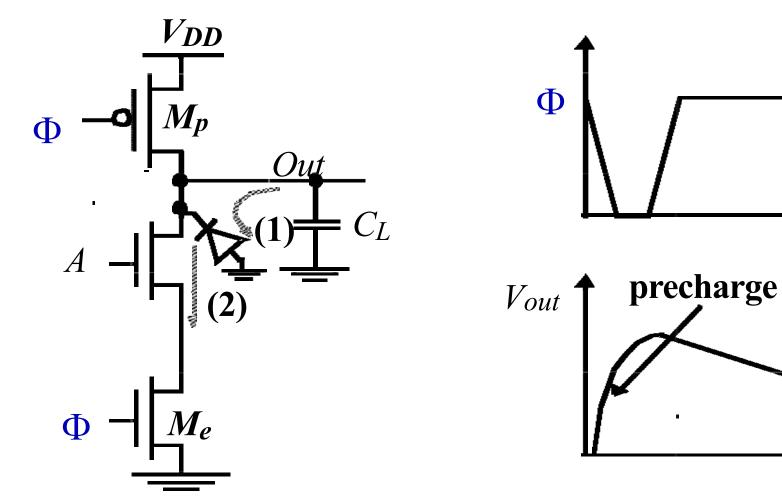
(a)Leakage sources (b) Effect on waveforms
