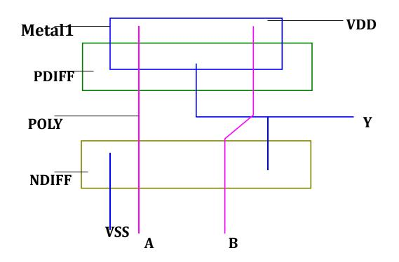
Symbol and Stick Diagram of 2 inputs NAND gate
