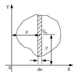
m.I is denoted by I and carries with it the symbol of the axis about which it is calculated. m.I of the strip about 0Y axis,  $I_{0Y}$  srip=  $area \times distance^2$
