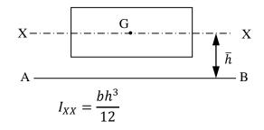
The moment of inertia of the same rectangle, about any axis, but parallel to XX axis can be determined by parallel axis theorem. Let AB is a parallel axis , parallel to XX, at a distance of  $\bar{h}$ . From parallel axis theorem
