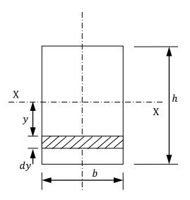
Consider a rectangle of base 'b' and height 'h' as shown in fig. Let us find the m.I of this rectangle about its centroidal axis XX and YY.
