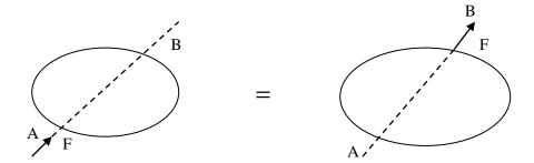
The condition of equilibrium or motion of a rigid body remain, unchanged if a force acting at a given point of the rigid body is replaced by a force of same magnitude and direction, but acting at a different point provided that the two forces have the same line of action.
