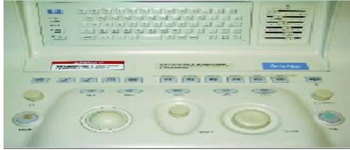
▲ An ultrasound console showing the time gain compensation sliders and the depth and gain controls. Names and locations of ultrasound controls vary from unit to unit.
