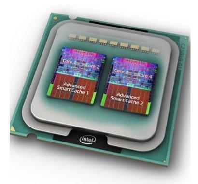
A dual-core configuration is comparable to having several different processors installed on the same computer, but the connection between them is faster because the two CPUs are plugged into the same socket. Several instructions in parallel may be executed by individual cores, boosting the speed of software built to make use of the architecture's unique features.
