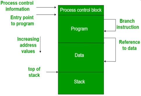
The figure depicts a process image. The process image is occupying a continuous region of main memory. The operating system will need to know many things including the location of process control information, the execution stack, and the code entry. Within a program, there are memory references in various instructions and these are called logical addresses.
