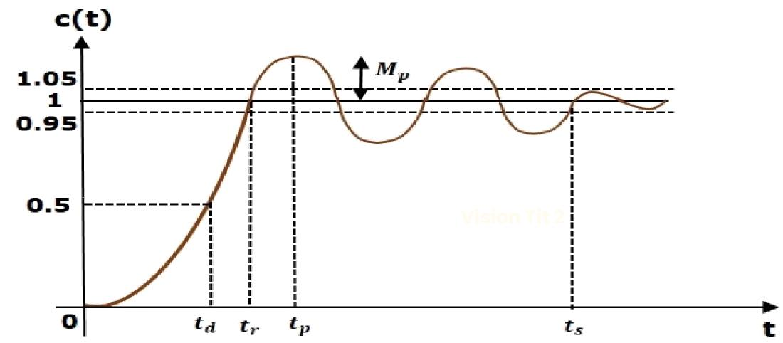
• It is the time required for the response to reach the peak value for the first time. It is denoted by  $t_p$  (sec). At  $t=t_p$ , the first derivate of the response is zero.
