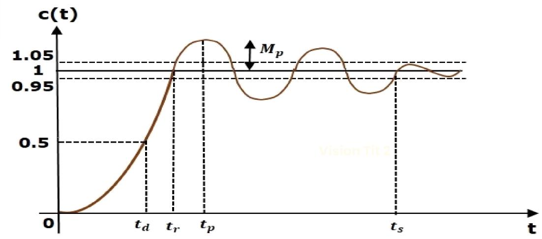
• It is the time required for the response to rise from 0% to 100% of its final value and represented by t<sub>r</sub> (sec)
