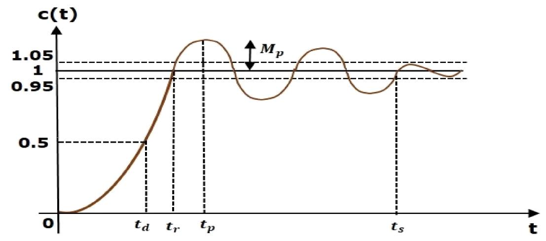
• It is the time required for the response to reach half of its final value from the zero instant. It is denoted by t<sub>d</sub> (sec)
