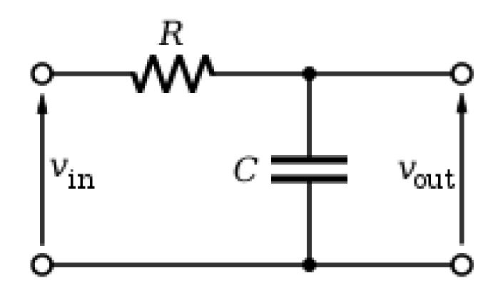
$$\frac{dV_{out}}{dt} = \frac{1}{RC}(V_{in} - V_{out})$$
