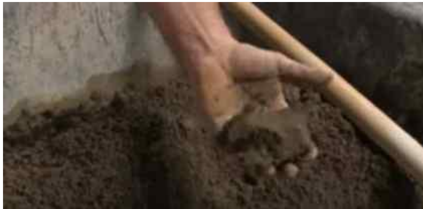
Fig. 1: Adequate Amount of Water Added
