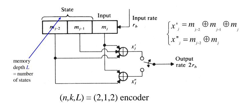
• Thus, for generation of n-bit output, we require in this example n shift registers in k = 1 convolutional encoder
