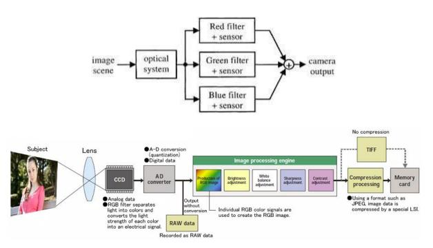
A digital camera's image quality is determined by three elements: lens performance, CCD image sensor pixel count and performance, and image processing engine performance.
