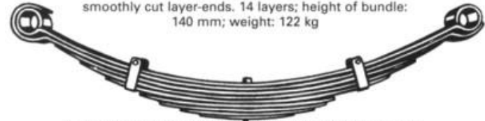
b. Improved multi-layered leaf spring with pressed layer-ends and plastic layers in between. 9 layers; height of bundle: 127 mm; weight: 94 kg
