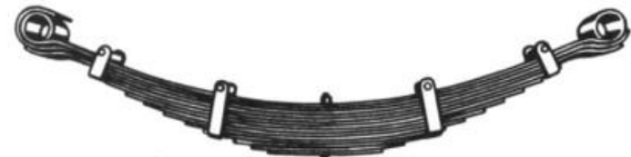
a. Conventionally multi-layered leaf spring with smoothly cut layer-ends. 14 layers; height of bundle: 140 mm; weight: 122 kg
