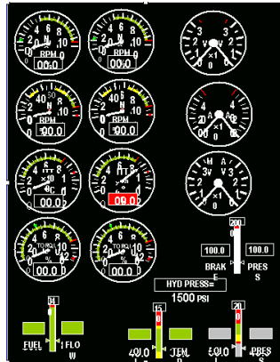
Fig. 7 Display Unit with typical symbology for EICAS
