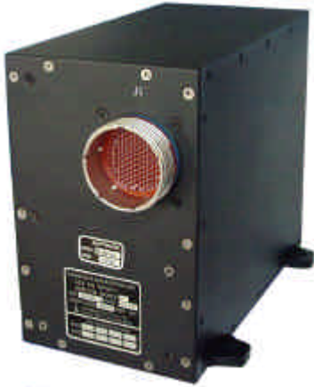
Fig. 6 Engine Data Concentrator Unit for EICAS
