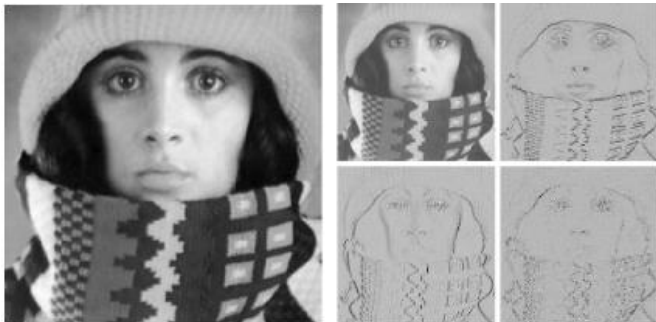
Decomposition of a grey-scale image by a morphological wavelet (max-lifting scheme). The original image is shown at the left and its decomposition into four subbands at the right.
