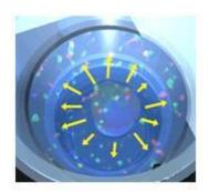
The energy of the solvent molecules is transferred to the fluor molecules, which in turn emit light
