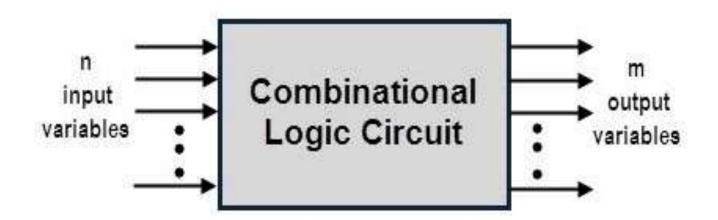
Combinational Logic Circuits are memoryless digital logic circuits whose output at any instant in time depends only on the combination of its inputs.
