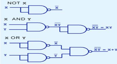
Three Circuits Constructed Using Only NAND Gates
